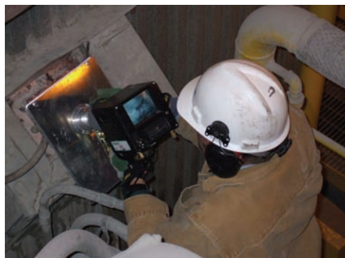
PyrOptix Mobile IR Camera in Use
