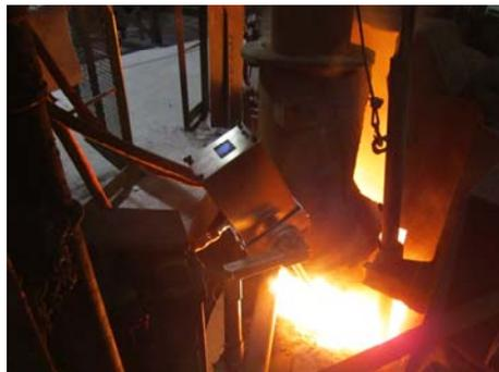
The PyrOptix ST fixed camera system is well-protected and provides unprecedented operational views of the Ladle Furnace, Basic Oxygen Furnace and Electric Arc Furnace. It also allows for an unobstructed view of the entire tapping process—virtually unaffected by dust, steam, arc flash, UV light or fireball.
